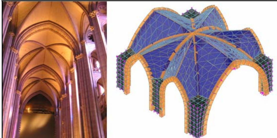
Figure 6. a) View of Nave Vaults of the Cathedral of St. John the Divine (NY), Showing Transverse Arches, b) The SAP 9.0 model of the vaults of the Cathedral of St. John the Divine in AutoCAD.
